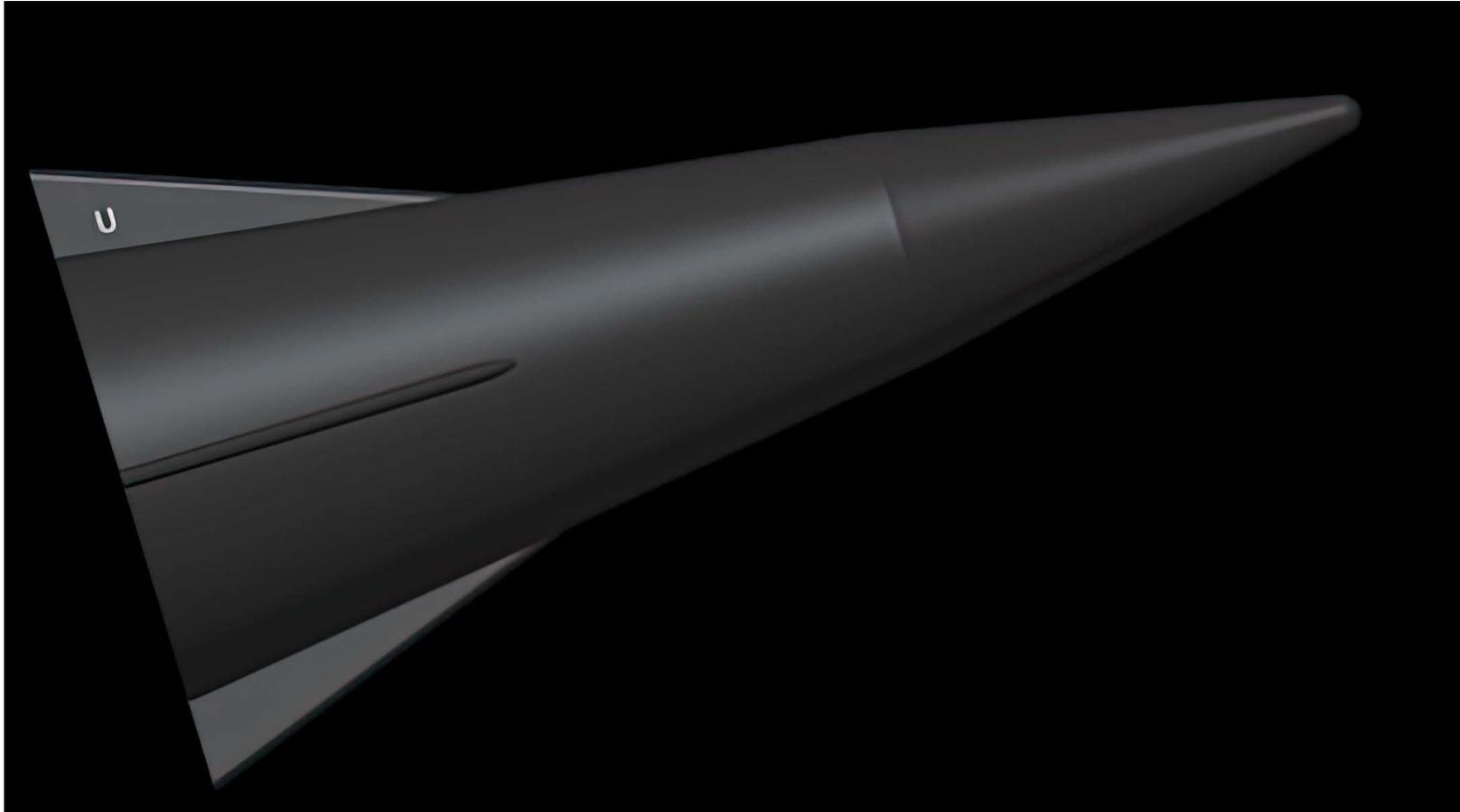
The Army and Navy are collaborating on the Common Hypersonic Glide Body (C-HGB), the part of a hypersonic boost-glide missile that detaches from the spent rocket booster and glides to its target. Both services plan to use the C-HGB in the hypersonic boost-glide missiles they are developing: the Army's Long-Range Hypersonic Weapon and the Navy's Intermediate-Range Conventional Prompt Strike missile.
