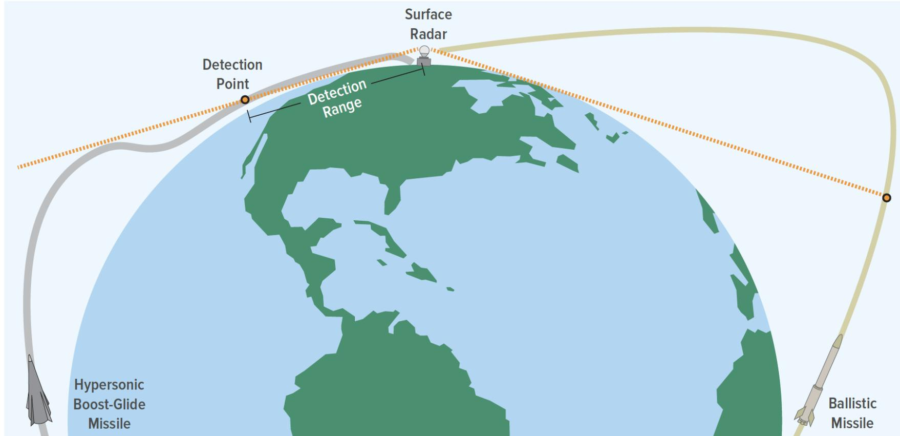
Because of the curvature of the Earth, a radar cannot detect a missile that is below the horizon. The distance to a radar's horizon increases with the height of the radar's antenna and the altitude of its target.
