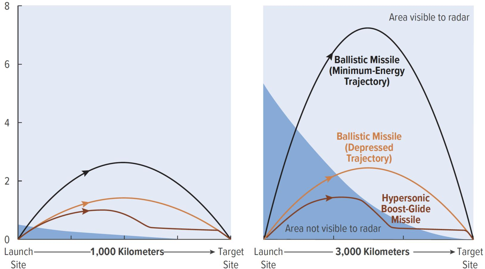
Because of its altitude, a ballistic missile would theoretically be visible to a radar located at the target site much earlier in its flight than a hypersonic boost-glide missile would be. To detect and track a missile, however, the radar would have to be powerful enough to generate a signal that would reach the missile.
