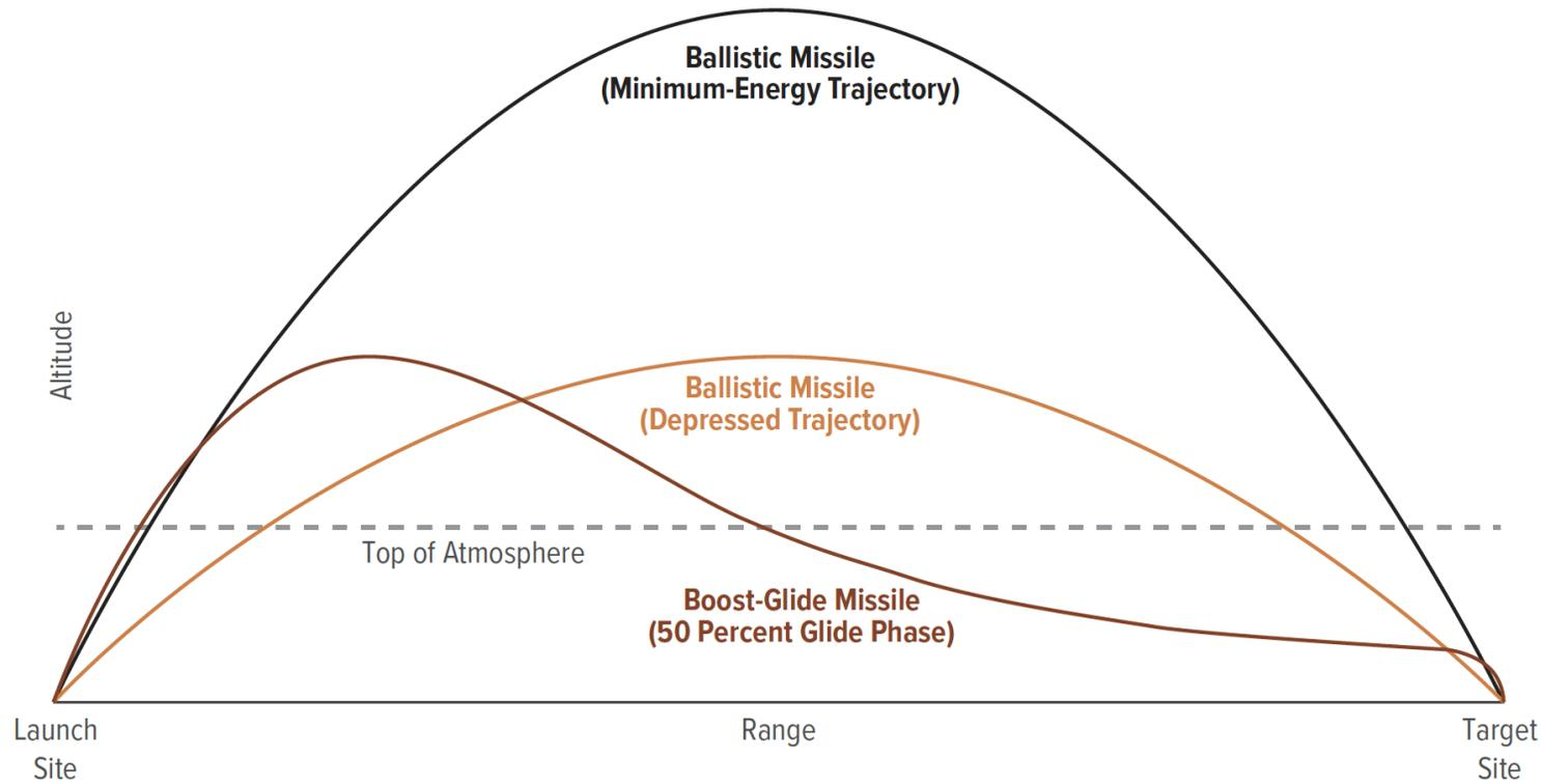
A missile's ballistic trajectory can be shaped in many ways. This figure shows a simple minimum-energy trajectory that is very close to a parabola, influenced mainly by gravity after the missile's rocket booster burns out, and a depressed trajectory, when the ballistic missile is launched at a shallower angle.
