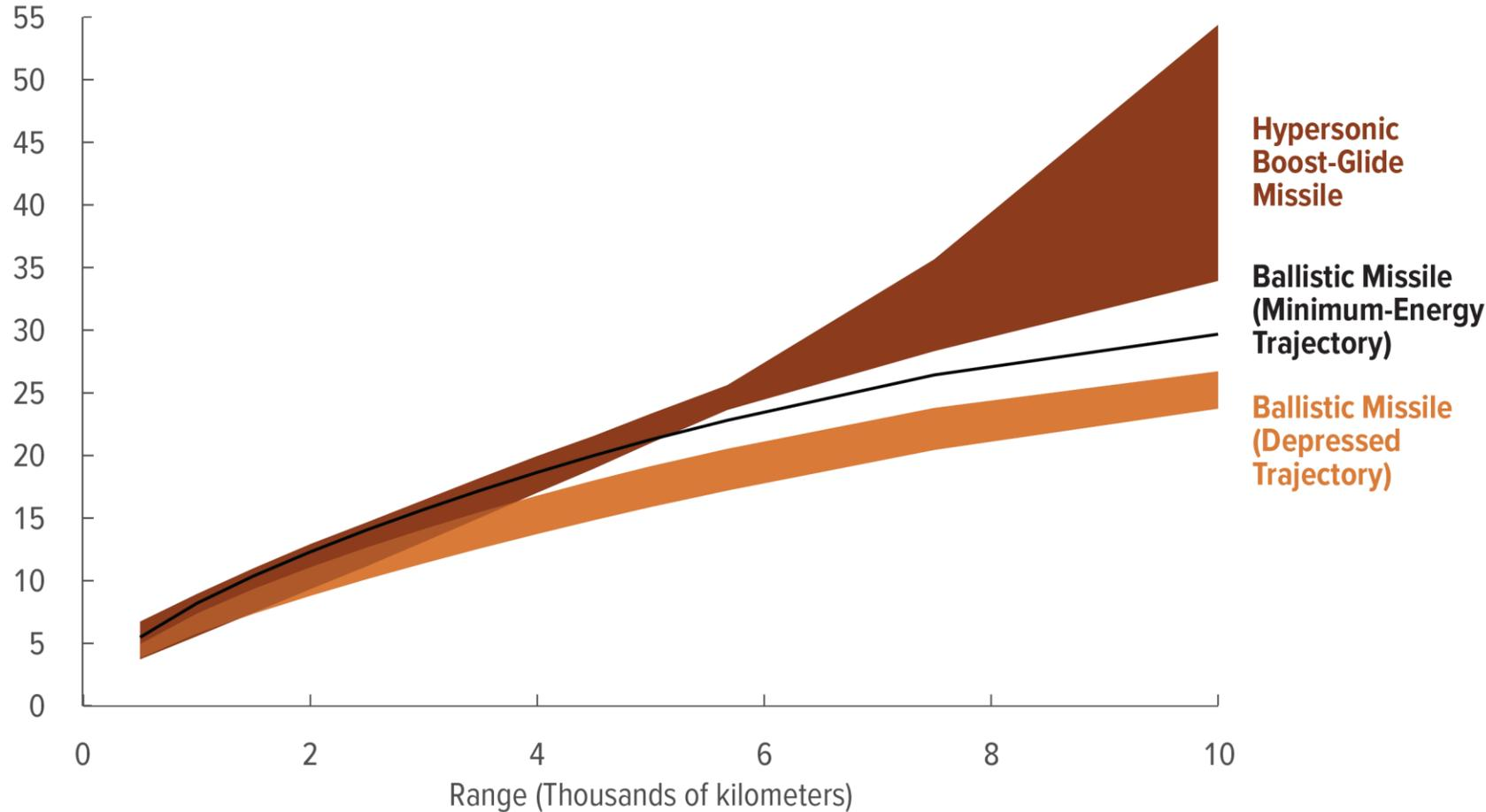
Currently planned hypersonic boost-glide missiles are likely to have longer flight times than ballistic missiles flying minimum-energy or depressed trajectories.
