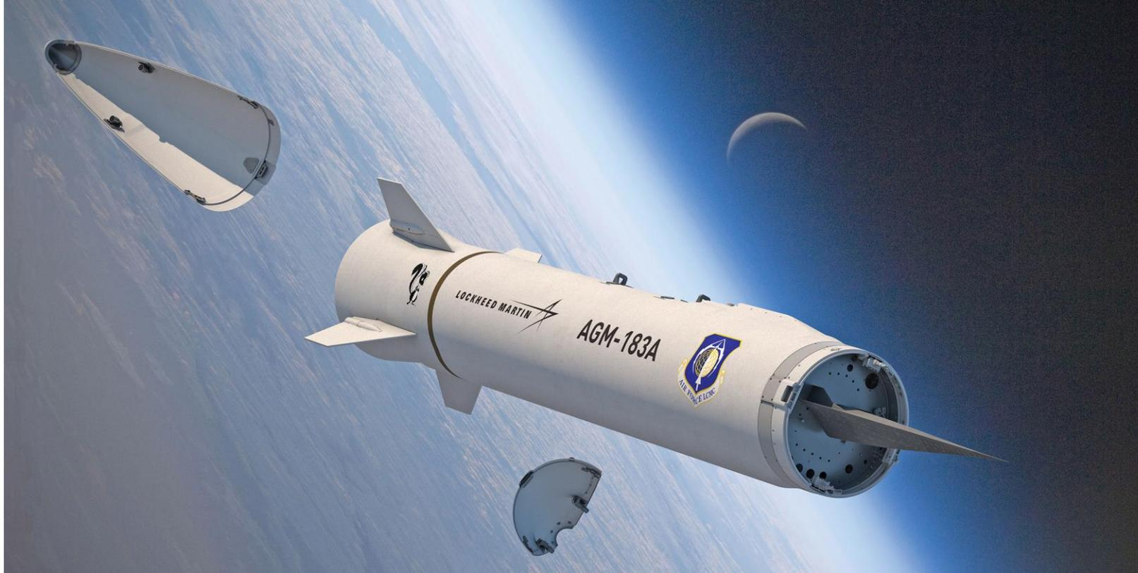
The Tactical Boost Glide (TBG) vehicle developed by the Defense Advanced Research Projects Agency forms the basis for the hypersonic boost-glide missile that the Air Force is developing, the Air-Launched Rapid Response Weapon. The TBG is shown here as a slender, pointed object on the front end of the missile. The cone in the upper left of the drawing is the protective shroud from the front of the missile, which has just been ejected in preparation for releasing the TBG.
