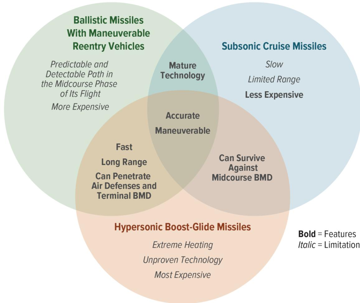
The hypersonic missiles being developed by the U.S. military combine desirable traits of two types of U.S. missiles with well-developed technology: ballistic missiles' speed and long ranges, and subsonic cruise missiles' maneuverability and ability to survive against midcourse missile defenses. Hypersonic missiles introduce new technical challenges, however.
