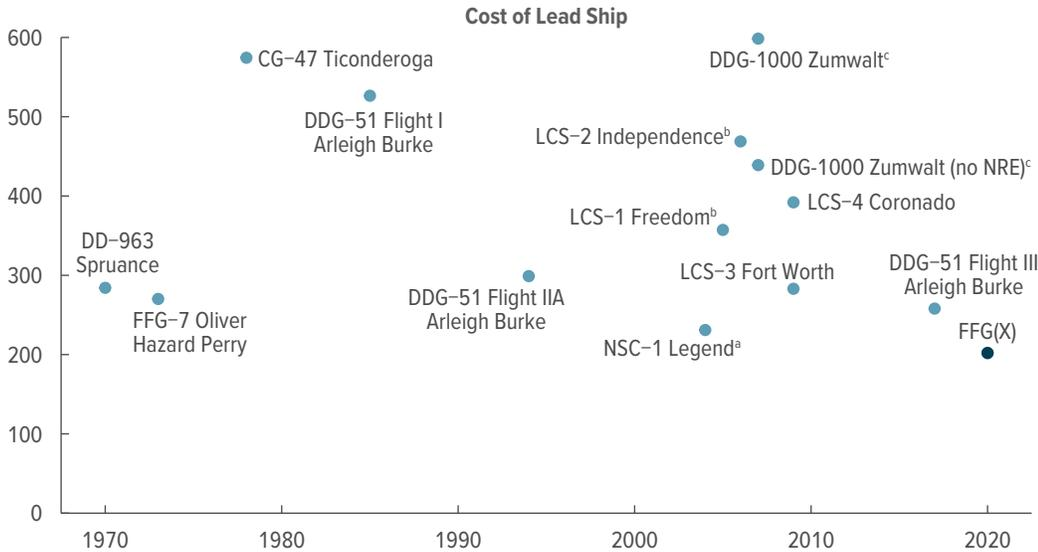
Every surface combatant built since 1970 cost more by weight to produce than the Navy expects its new FFG(X) frigate to cost.
