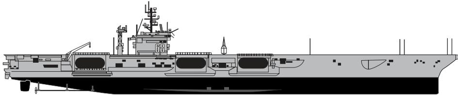
The Navy's 10 **aircraft carriers** are the heart of the battle force. Each carries an air wing of about 60 aircraft, which can attack hundreds of targets per day for up to a month before needing to rest. Carriers are the largest ships in the fleet, with a displacement of about 100,000 tons. All 10 current carriers belong to the Nimitz class.
